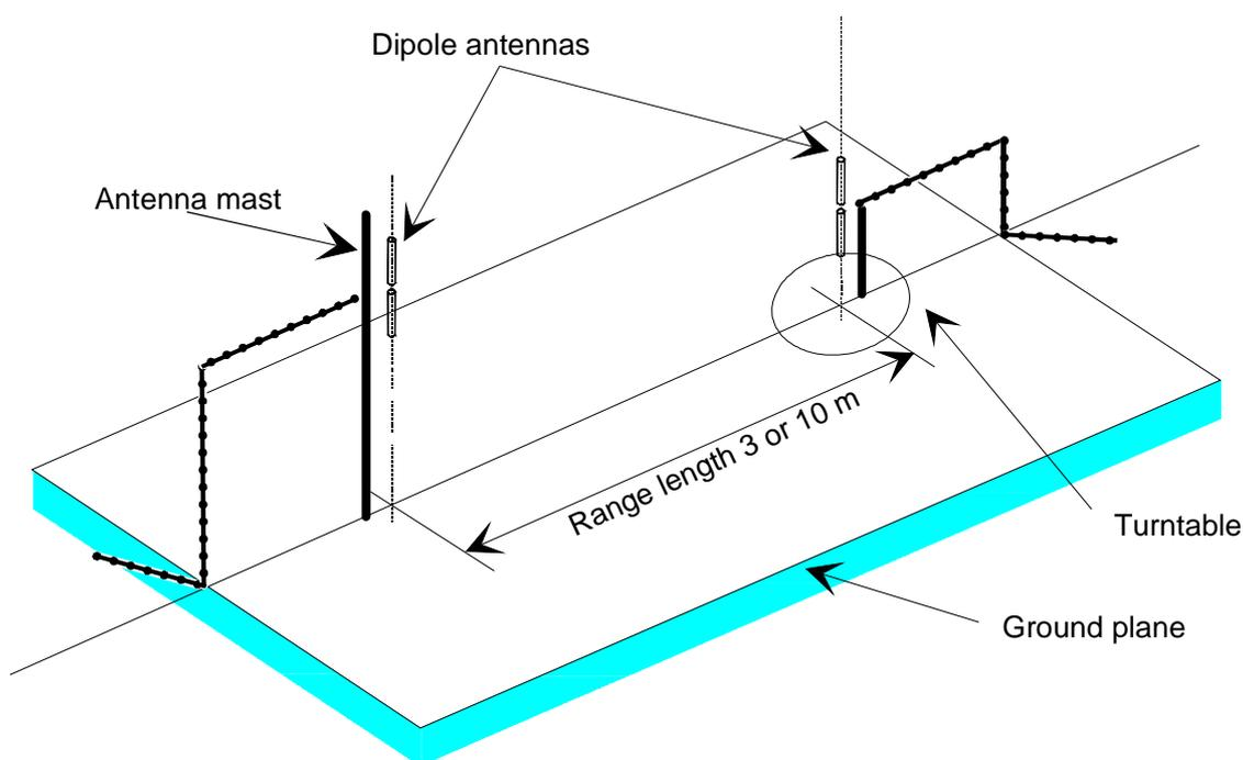
**Figure C.3: A typical Open Area Test Site**
